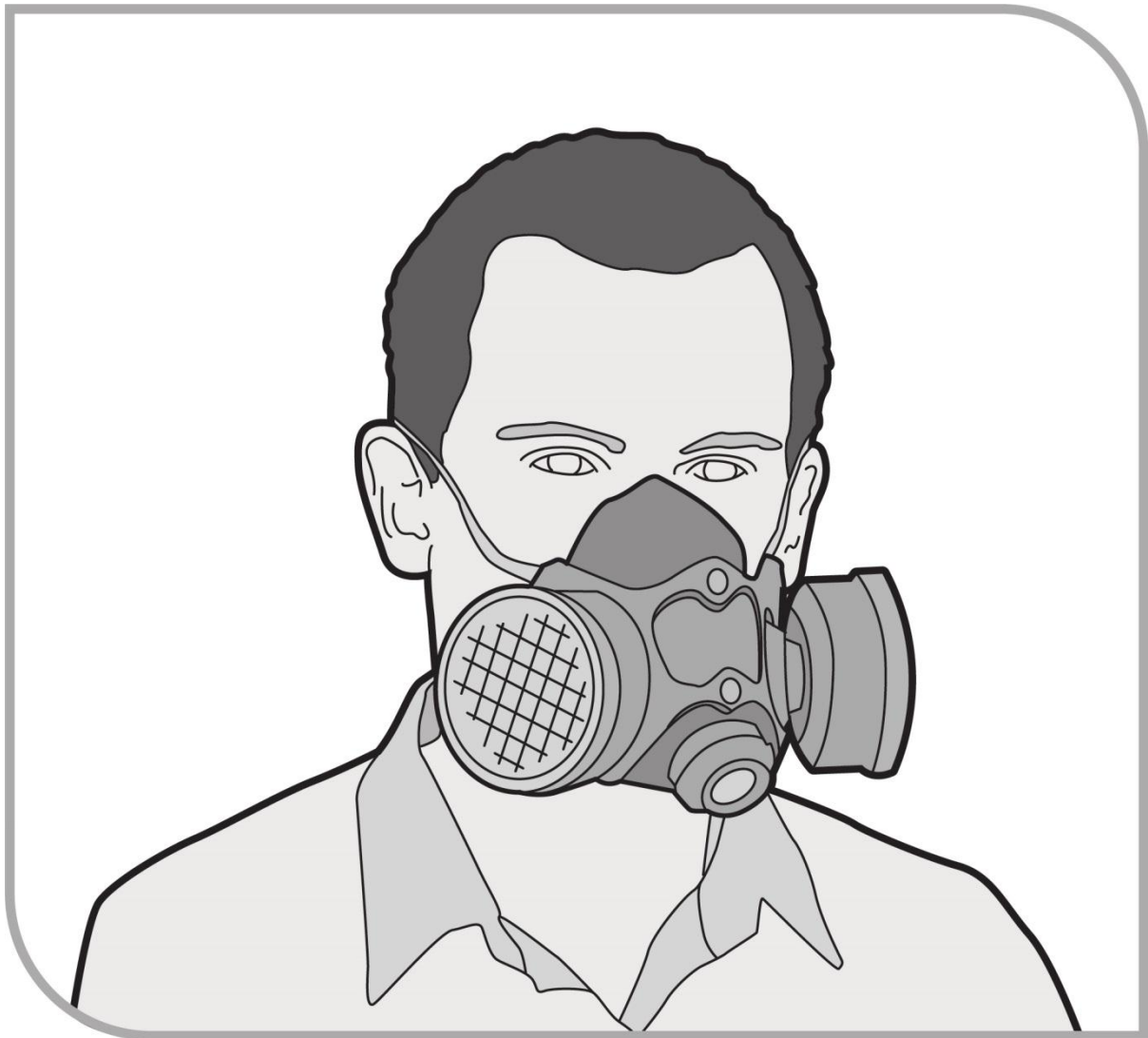
Figure 10 Half-face particulate filter (cartridge) respirator
