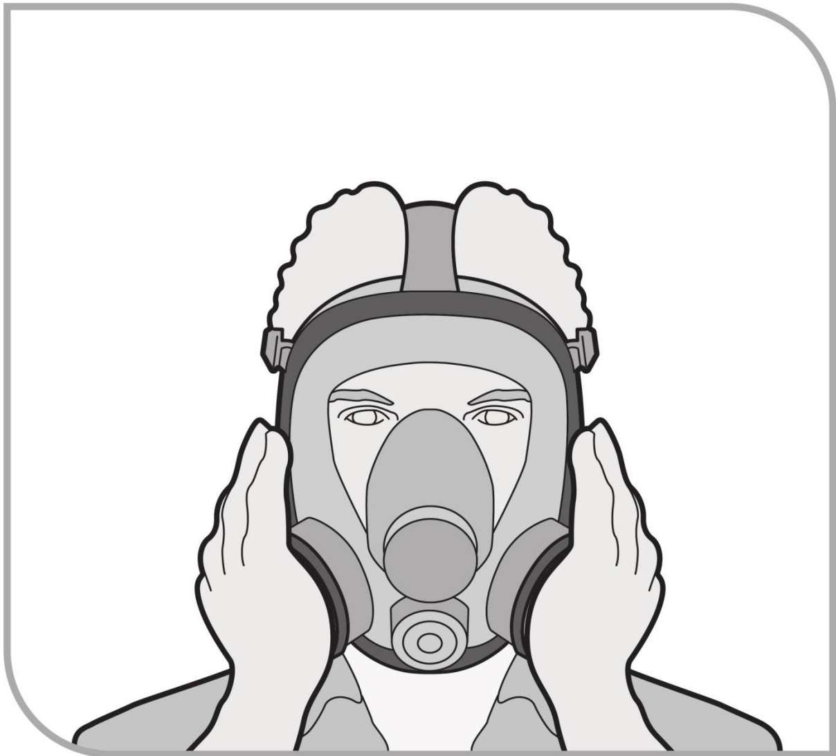
Figure 15 Conducting a fit check for a full-face, particulate filter (cartridge) respirator
