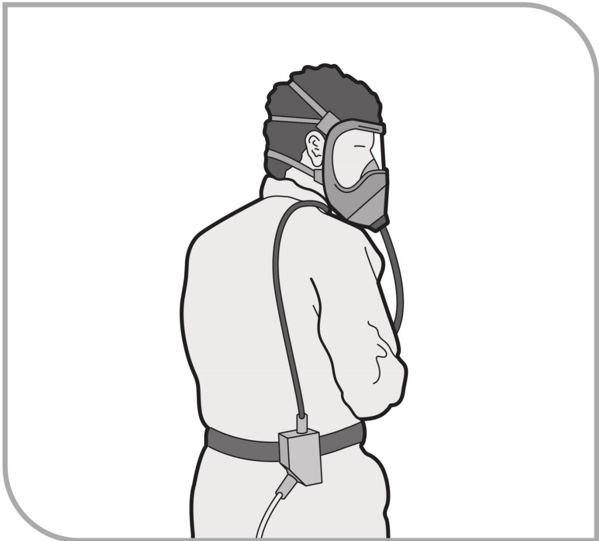
Figure 14 Full-face, positive pressure demand air-line respirator
