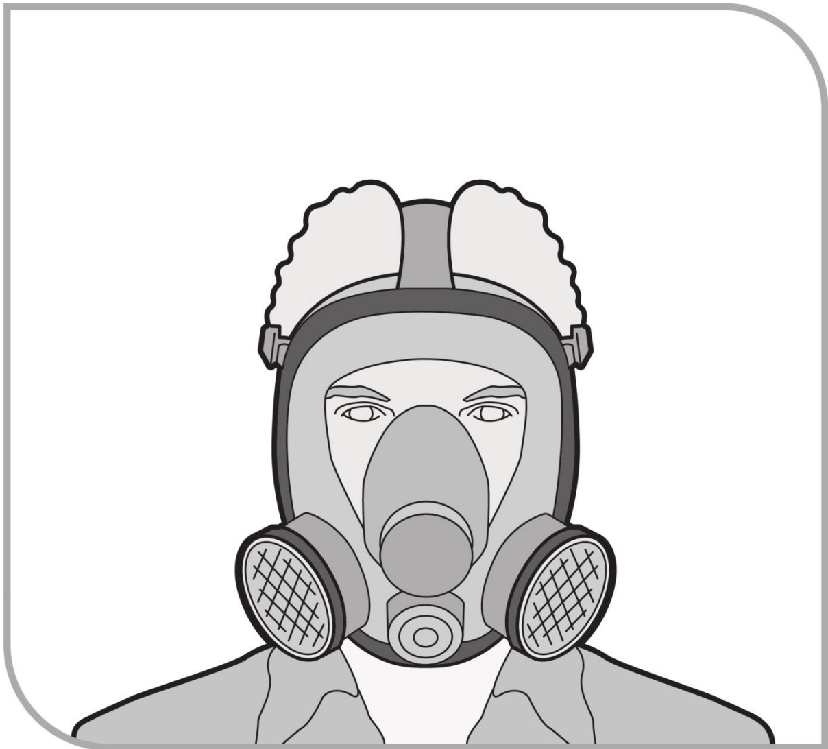
Figure 12 Full-face, particulate filter (cartridge) respirator
