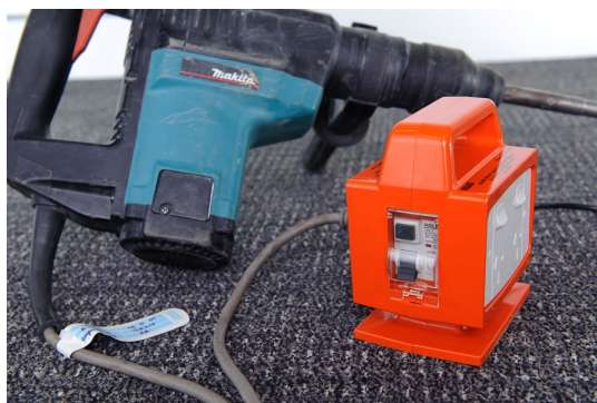
Figure 66 – Tested tag on LV portable electrical tool protected by an RCD
