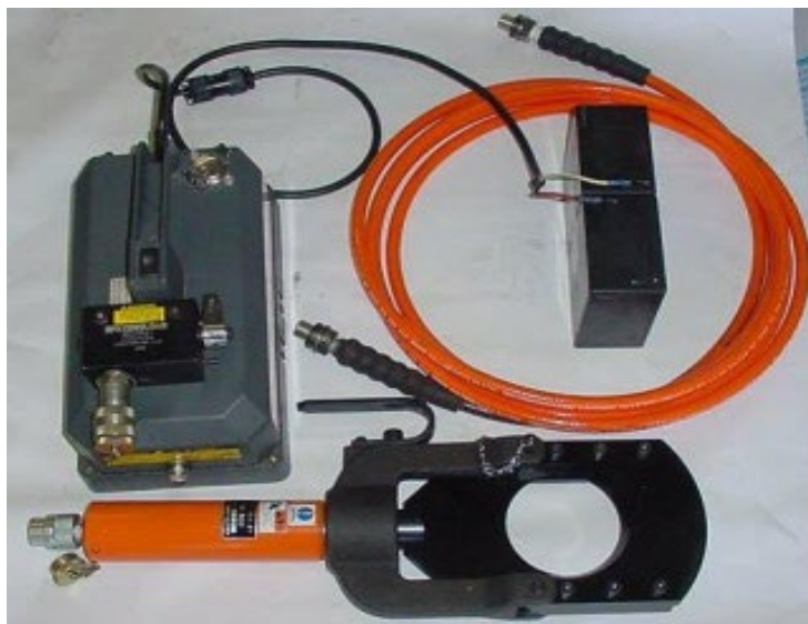
Figure 73 – Remote cable cutting equipment
