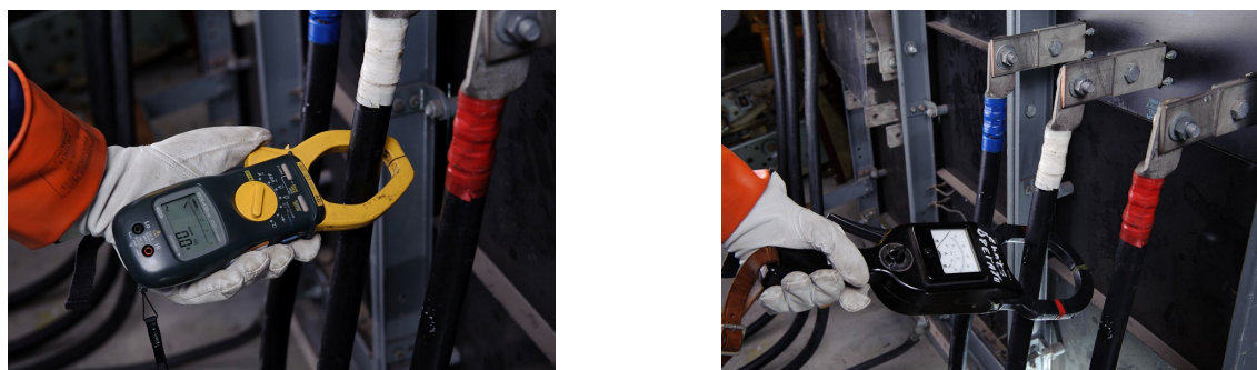
Figure 129 - Two types of tong ammeters used to measure current
