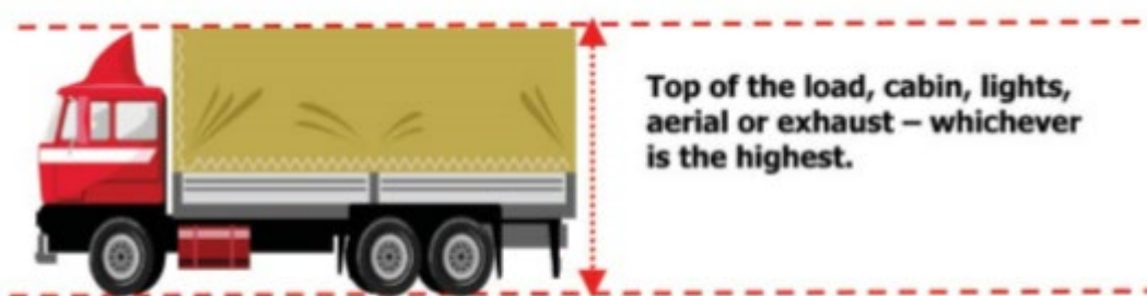
Figure 76 – An illustration of the maximum overall height of a vehicle (Image courtesy of SafeWork NSW)
