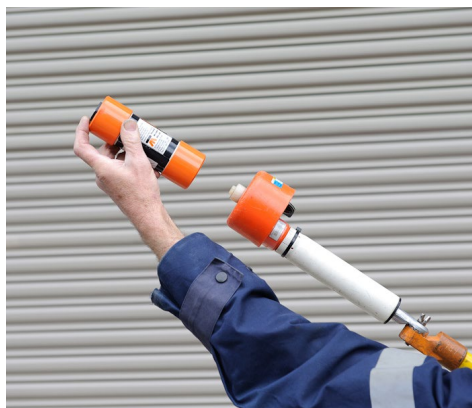
Figure 106 - Checking HV detector
