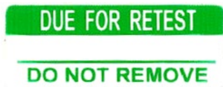
Figure 69 – An example of a test sticker for HV insulated tools
