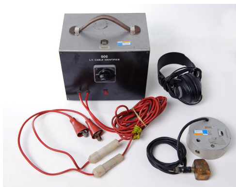
Figure 71 - Live LV cable identification equipment
