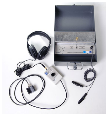
Figure 72 - Cable identification generator and receiver
