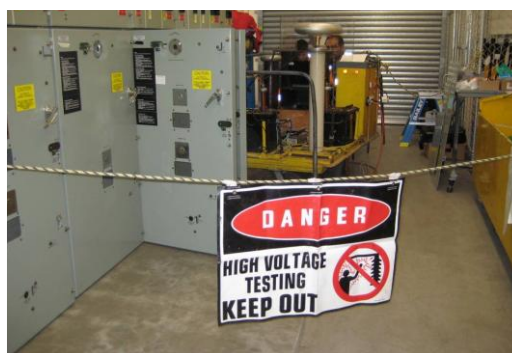
Figure 90 - Black and yellow rope barrier with danger notice
