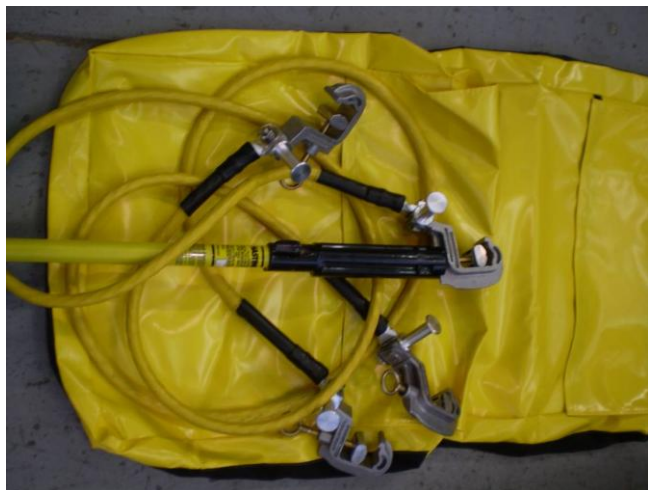
Figure 77 – Portable earthing and short-circuiting equipment
