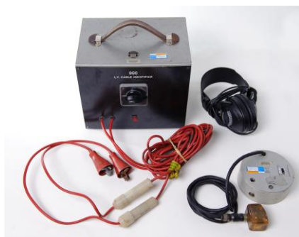
Figure 27 - Live LV cable identification equipment
