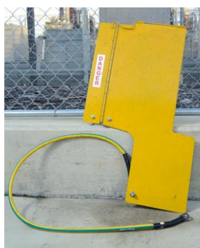
Figure 31 – An earthed screen for Hazemeyer switchgear
