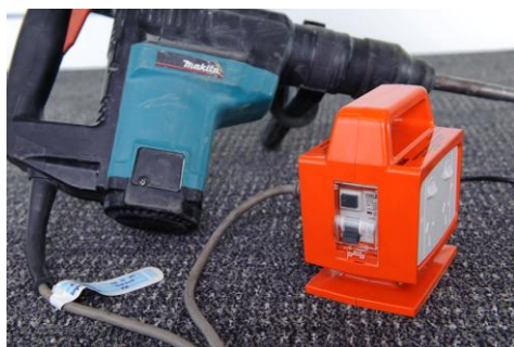
Figure 39 – Tested tag on LV portable electrical tool protected by an RCD
