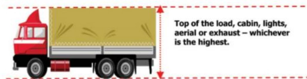
Figure 43 – An illustration of the maximum overall height of a vehicle (Image courtesy of SafeWork NSW)
