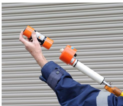
Figure 75 - Checking HV detector
